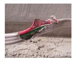
If you find conditions which may be a danger to people in a public place (such as damaged live mains and apparatus, fallen mains, leakage current on poles, etc), you must initially remain well clear of the mains and apparatus, but in a position to warn people until the danger has been removed. If you cannot do this, you must arrange for another responsible person to do so.
