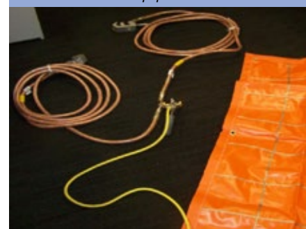
Fault current bypass cable assembly after connection to equipotential earth mat.
