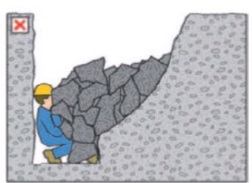
Figure 4: The worker is crushed against the opposite excavation wall by the collapsing ground. It should be noted that the weight of a wedge of sand 1m x 2m is approx. 3 Tonnes.
